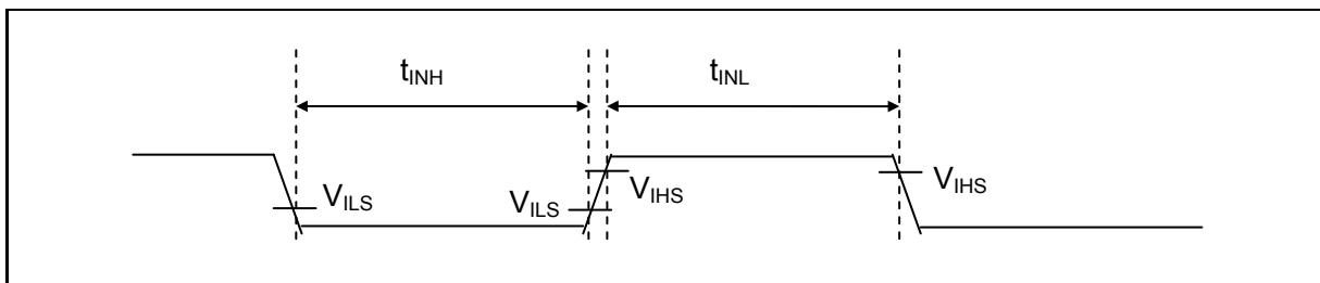
(10) I<sup>2</sup>C timing(V<sub>CC</sub> = AV<sub>CC</sub> = DV<sub>CC</sub> = 2.7V to 5.5V, V<sub>SS</sub> = AV<sub>SS</sub> = DV<sub>SS</sub> = 0V, T<sub>A</sub> = -40°C to +105°C)
